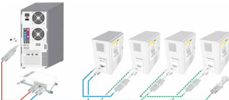
Extendable for connection of up to 16 furnaces
